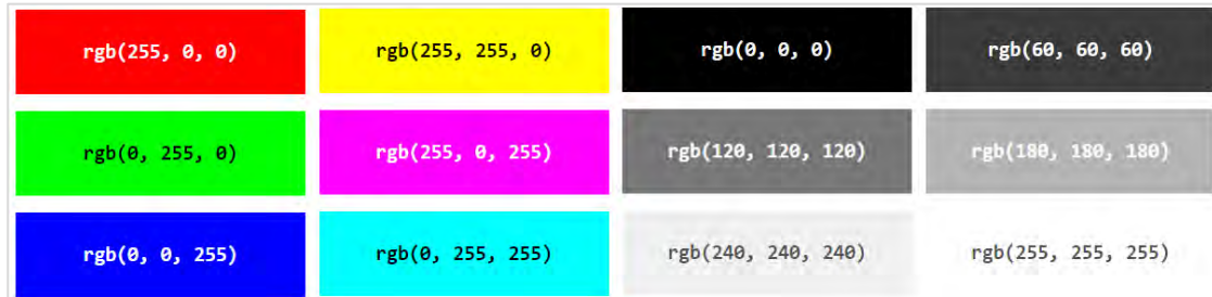
Fig. 13: The rendering of the primary colours and those resulting from their addition on digital devices.
